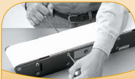
Rack and Pinion Belt Tensioning
