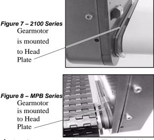
**4.** Attach mount assembly (I of Figure 9) with two screws (O). Tighten screws to 80 in-lb (9 Nm).
