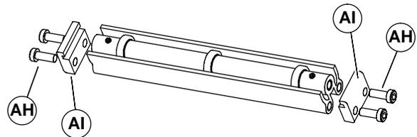
2. Remove screws (AH of Figure 16) and clips (AI) from roller assembly.
