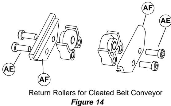
2. Remove screws (AE of Figures 13 & 14) and clips (AF) from roller assembly.
