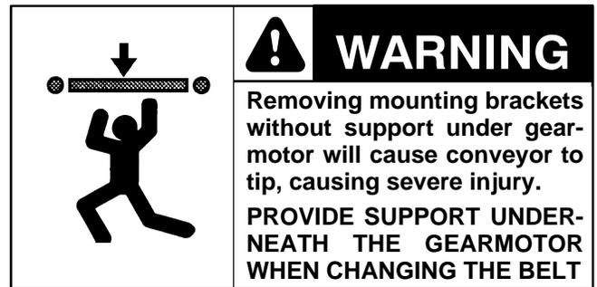
1. Place temporary support stands (BO of Figure 37) at both ends of the conveyor. See WARNING.
