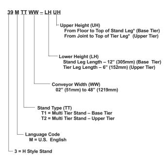
\* When raised to its maximum height, top of conveyor mounting bracket (Figure 1, item F) is at the same height as top of stand leg (D) (base tier) or tier leg (B) (upper tier).
