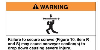
TIGHTEN SCREWS (R and S) AFTER ADJUSTMENT.
