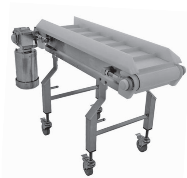
Cleated Belt Conveyor
