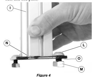
**4.** Align the leg tube end plate hex nuts (M of Figure 5) with the t-slots (P) on one side of the trileg post (G). Slide the hex nuts (M) into the T-slots (P).
