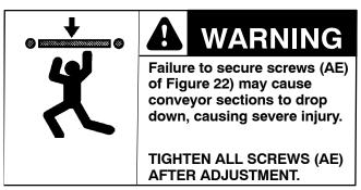
9. Tighten fastening hardware (AE of figure 22) to 100 in-lb (11 N-m).
