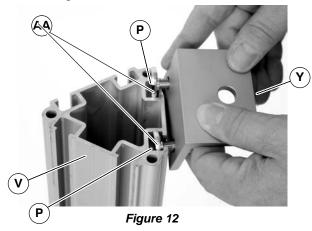
**5.** Align the foot bracket edge (Y of Figure 13) with the bottom edge of the trileg post (V).
