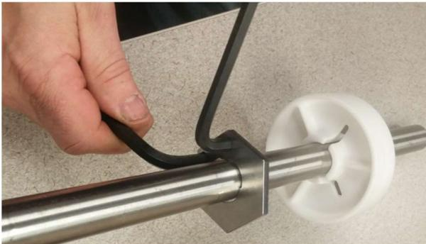
5. Rotate larger wrench 30 degree away from smaller wrench – closing clip and clamping on shaft.
