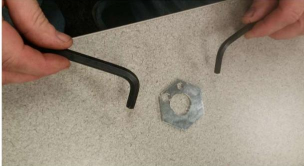
3. Insert 6mm or 1/4" hex key wrench in smaller hex hole and 8mm or 5/16" hex key wrench in slotted hex hole with arms pointing away from center hole. Rotate larger wrench 30 degree towards smaller wrench – opening clip.
