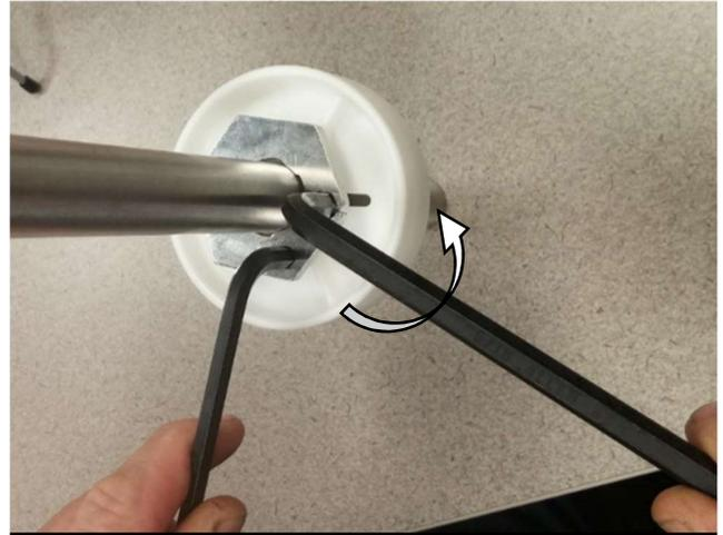
6. Remove hex wrenches and ensure roller spins freely. If necessary adjust location.
