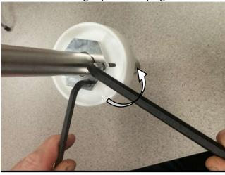
6. Remove hex wrenches and ensure roller spins freely. If necessary adjust location.
