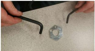
3. Insert 6mm or ½" hex key wrench in smaller hex hole and 8mm or 5/16" hex key wrench in slotted hex hole with arms pointing away from center hole. Rotate larger wrench 30 degree towards smaller wrench – opening clip.
