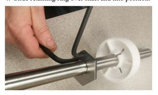
5. Rotate larger wrench 30 degree away from smaller wrench – closing clip and clamping on shaft.
