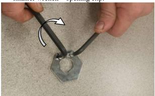
4. Slide retaining ring over shaft and into position.
