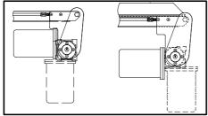
Figure 3: Gearmotor Re-orientation Details for Flat Belt Conveyor (left) & Cleated Belt Conveyor (right)
