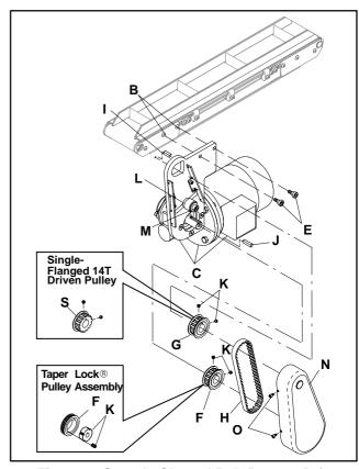
Figure 4: Sample Cleated Belt Bottom Drive
