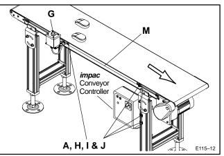
Figure 12: Jog Cable Routing to impac Conveyor Controller
