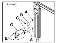
Figure 7: Jog Horizontal Mounting to Aluminum Stand Leg
