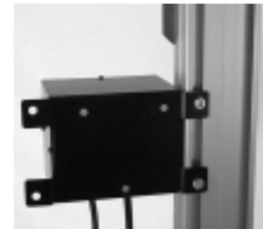
**Step 3:** Using screwdriver, raise 2nd T-bar to align it with upper mounting tab hole and insert a screw (D) and partially thread into T-bar as shown. Then position controller to desired location and tightly secure both screws (D).
