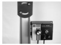
DC Controller Attached to Aluminum Stand
