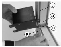
Step 1: Place 1st T-bar (G) into T-slot, insert screw (D) into hole in lower mounting tab and, using a 4 mm hex key wrench, partially thread into T-bar.
