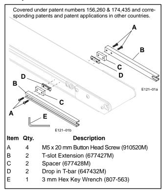
Figure 1: T-slot Extension Kit (307000M) Parts
