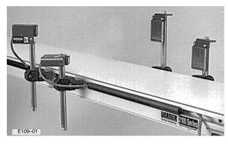
Figure 1: Photo-Eye Kit Installed (75-31)
