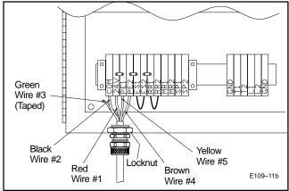
Figure 11: Sample Photo-Eye to impac Wiring Connections
