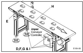
Figure 9: Photo-Eye Cable Routing to impac Conveyor Controller
