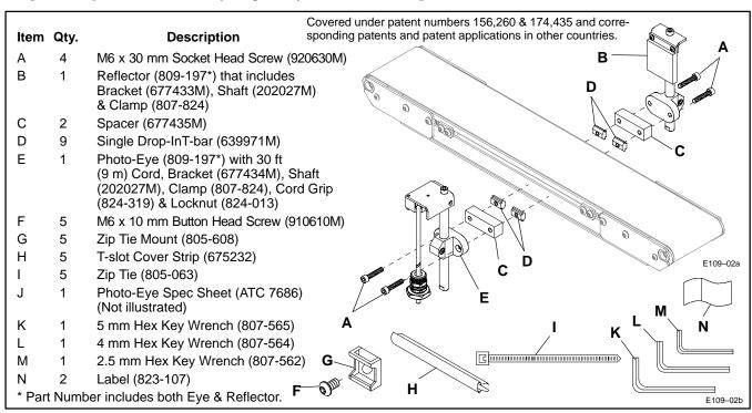
Figure 2: Photo-Eye Kit (75-31) Components
