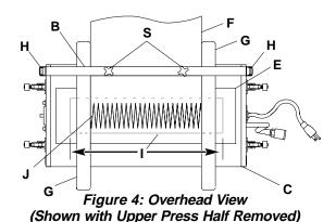
4. Place the one end of the belt (F of Figure 4) onto the teflon release fabric (E) so that the splice fingers (J) are horizontally and vertically centered as shown. Next, lay the appropriate thickness (see Table 1) shims (G) against the belt, with equal amounts extending beyond each side of the press as shown. Then, attach the clamping bar (B) by engaging the latches (H). Be sure that the shims are tight against the sides of the belt before tightening the clamping bar knobs (S).
