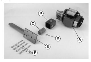
Step 3: Build gearmotor assembly as shown. Tighten screws (F) with 50 in-lb (5.6 Nm) of torque. NOTE: Refer to the following drawing for alternate motor positions.
