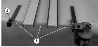
Step 12: Slide hex shaft through conveyors and into flex coupling while placing shaft cover (I) pieces between components.
