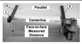
Step 4: Attach the gearmotor support assembly (E) and bearing support assembly (G) to their respective mounting surfaces.
