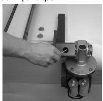
Step 14: Secure the coupling to hex shaft by tightening both set screws. Visually inspect coupling for correct alignment (equal gaps in coupling grooves). Replace access plugs.
