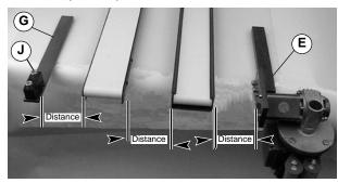
Step 7: Properly align and position conveyors between gearmotor support assembly (E) and bearing support assembly (G) as required. Do not secure the conveyors to the mounting surface.
