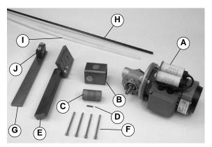
Step 1: Layout the gearmotor assembly and all loose parts as shown.
