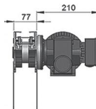
Located in middle section of conveyor to free up drive end.
