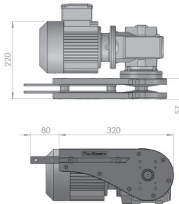
Note: Drive Module is 12 mm wider than conveyor frame.
