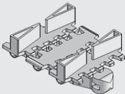
The above chain is FMCT-5A17-L1, 1 link cleated top chain with alternate of 1 link of plain chain.
