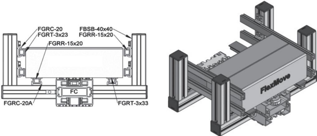
Width Adjustment Guide Rail Assembly      Packaging Box Handling
