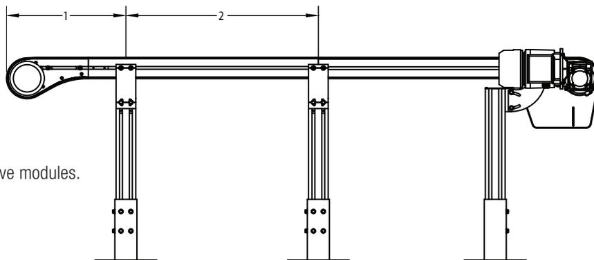
Support must be provided directly at drive end. See accessories for Direct Mount and Suspended Mount support options.
