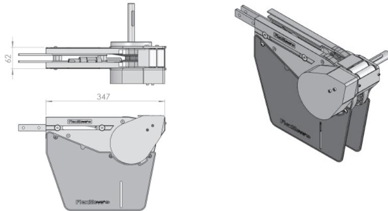
Note: Drive Module is 12 mm wider than conveyor frame.
