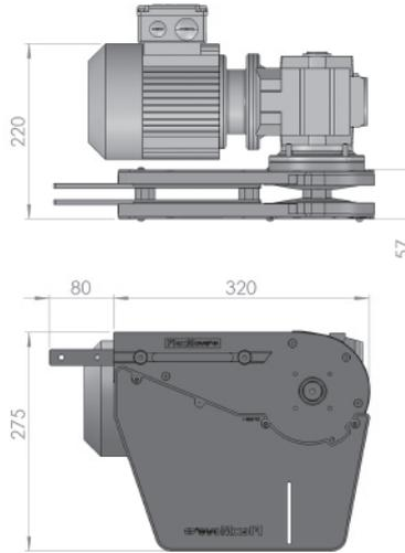
Note: Drive Module is 12 mm wider than conveyor frame.
