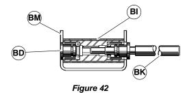
**8.** Insert sleeve arbor tool (BK of Figure 43) into opposite side of conveyor.
