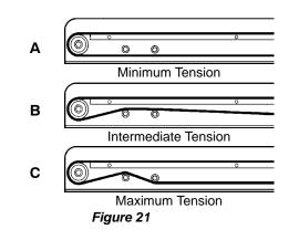
1. Locate tension versus conveyor belt as required for tension setting (A, B or C of Figure 21). Insert tension pin assembly (AL of Figure 22) into conveyor frame through hole (AM).
