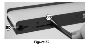
7. Insert pulley installation tool (BQ of Figure 53) into opposite side of conveyor and push retaining sleeve (BD) into pulley until flush with conveyor frame.
