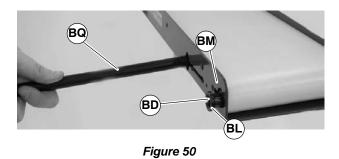
5. Insert pulley installation tool (BQ of Figure 51) into opposite side of conveyor.
