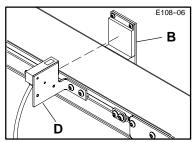
Figure 6: Photo-Eye & Reflector Alignment
