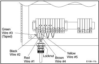
Figure 11: Sample Photo-Eye to impac Wiring Connections
