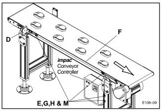
Figure 9: Photo-Eye Cable Routing to impac Conveyor Controller
