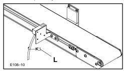
Figure 10: Cable Labeling (Detail provided only on Photo-Eye End of Cable)
