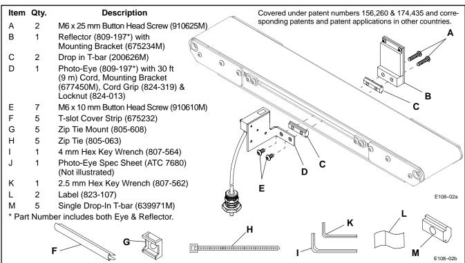
Figure 2: Photo-Eye Kit (75-30) Components
