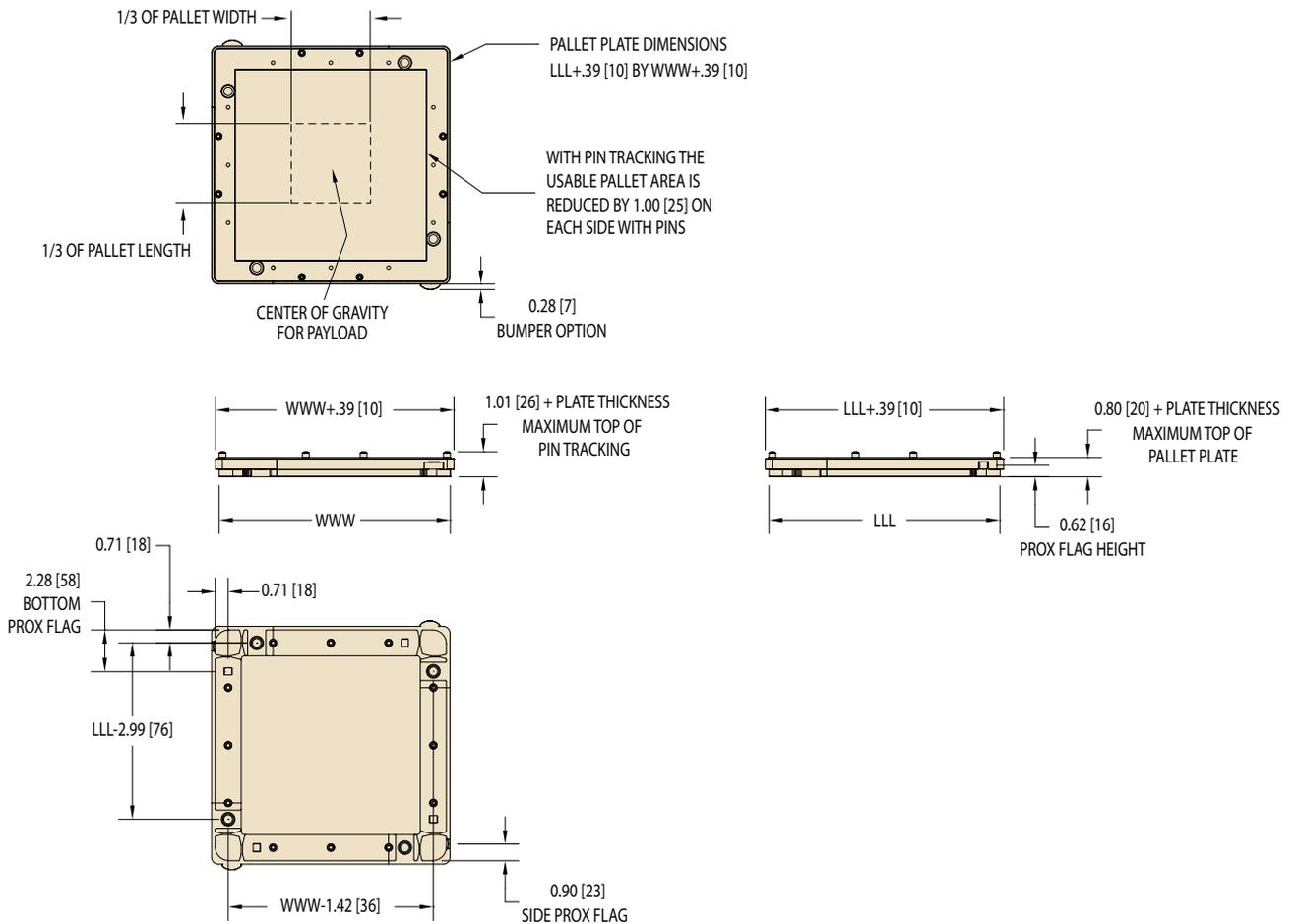
See page 54 & 58 for detailed pallet weights and detailed pallet plate drawings.
