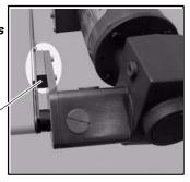
**4a.** Locate drive mounting position and remove two (2) screws (J of Figure 7).
