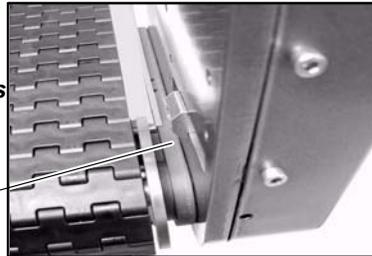
4. Attach mount assembly (I of Figure 9) with two screws (O). Tighten screws to 80 in-lb (9 Nm).
