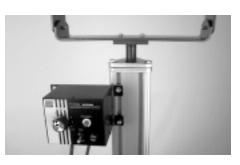
DC Controller Attached to Single Post Support Stand Figure 6
