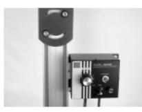
DC Controller Attached to Aluminum Stand Figure 7
