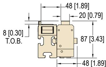
Part Number DS2SM-SFx where x: **N** = no sensor, **B** = Bottom sensor, **S** = side sensor
