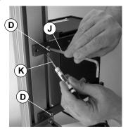
Step 3: Using screwdriver, raise 2nd T-bar (E) to align it with hole in the top mounting bar and insert a screw (D) and partially thread into T-bar as shown.
