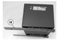
Step 1: Remove cover by loosening mounting screws (I). Then, properly orient and attach the mounting bars (H) in the "stand leg mounting" position. Attachment details similar to Step 1 on opposite side of this page.
