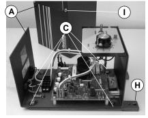
Step 1: Remove cover by loosening mounting screws (I). Use mounting screws (C), to attach mounting bars (H) as shown.
