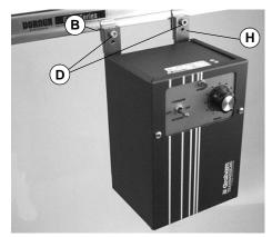
Step 3b: Secure box to 6100 Series conveyor by installing M6 Screws (D) through holes in mounting bars (H) and into accessory clips (B).
