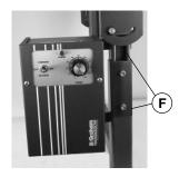
Step 1: Properly orient and install spring nuts (G) as shown. Then, secure controller by installing two (2) M6 x 25 screws (F). Adjust controller position and secure the M6 screws.
