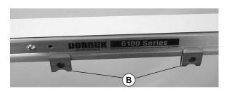
Step 2b: Accessory clips positioned on 6100 Series conveyor.
