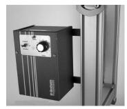
Step 4: Slide controller to its desired mounting location and tightly secure both screws (D).
