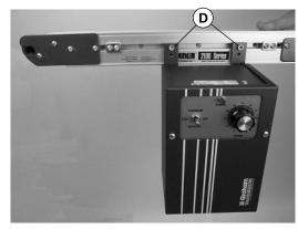
Step 3a: Secure box to 2100 Series conveyor by installing M6 Screws (D). (3100 Mounting Similar)
