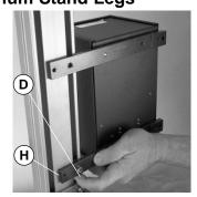
Step 1: Install 1st T-bar (E), insert screw (D) through hole in bottom mounting bar (H) and, using 4 mm hex key wrench, partially thread into one T-bar.
