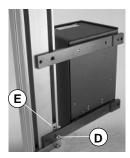
Step 2: Temporarily fix controller mounting position by tightening screw (D). Then, insert 2nd T-bar (E) into T-slot as shown.
