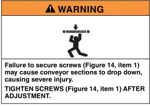
3. Secure flange socket screws (**Figure 14**, **item 1**) to 24 ft-lb (18 Nm).
