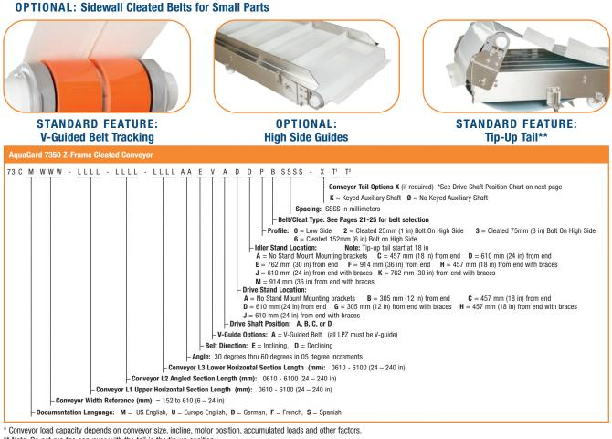
\*\* Note: Do not run the conveyor with the tail in the tip-up position.
