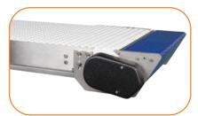
**OPTIONAL: Powered Transfer** For small parts and maintaining speeds through transfer. Series driven with speeds up to 78.6 m/min (260 ft/min). Transfer parts as short as 75 mm (3 in) long.
