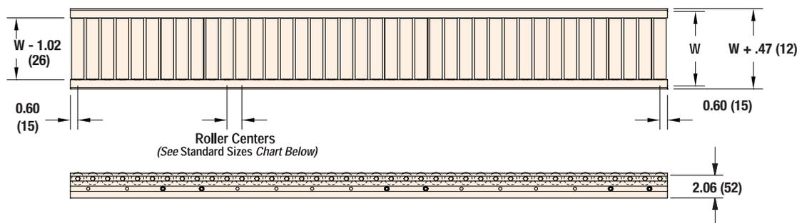
\* All conveyors are shipped with a roller at each end. Depending on roller centers, one odd roller space may occur. All frames are punched for rollers 0.6" (15) from each end on 1.2" (31) centers.
