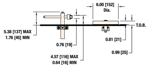
Pulley Transfer Plate (2200 Belted Conveyor Only)
