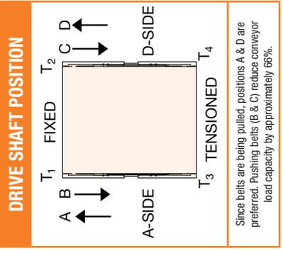
Since belts are being pulled, positions A & D are preferred. Pushing belts (B & C) reduce conveyor load capacity by approximately 66%.
