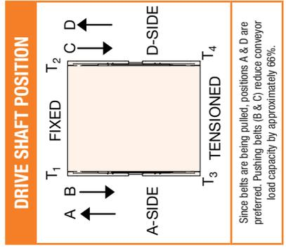
Since belts are being pulled, positions A & D are preferred. Pushing belts (B & C) reduce conveyor load capacity by approximately 66%.
