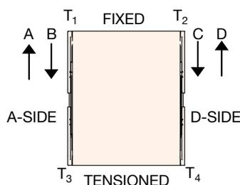
Since belts are being pulled, positions A & D are preferred. Pushing belts (B & C) reduce conveyor load capacity by approximately 66%.
