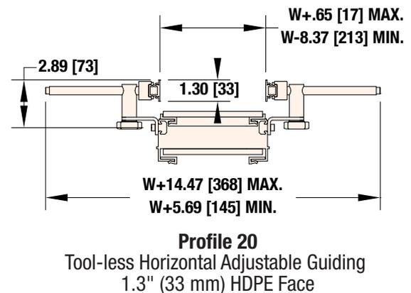
W = Conveyor Belt Width Dim = in (mm)
