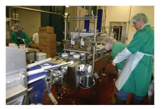
Designed solely for food, pharmaceutical and other industries that require conveyor systems with a high level of sanitation, the conveyor can be disassembled and cleaned in a matter of minutes.
