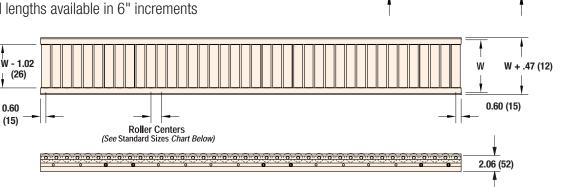
\* All conveyors are shipped with a roller at each end. Depending on roller centers, one odd roller space may occur. All frames are punched for rollers 0.6" (15) from each end on 1.2" (31) centers.
