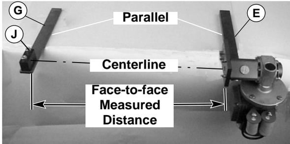
**Step 4:** Attach the gearmotor support assembly (E) and bearing support assembly (G) to their respective mounting surfaces.
