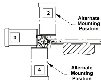
**NOTE:** Position "4" may reduce gear reducer oil seal life.
