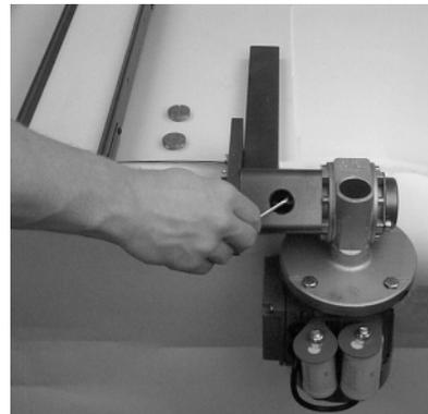
**Step 14:** Secure the coupling to hex shaft by tightening both set screws. Visually inspect coupling for correct alignment (equal gaps in coupling grooves). Replace access plugs.
