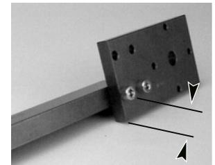
**Step 2:** Verify that factory-configured gearmotor support assembly is correct for your conveyor model - 2100 setup (left) and 4100 or 6100 setup (right).
