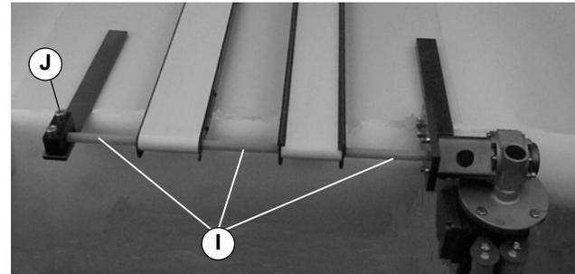
**Step 12:** Slide hex shaft through conveyors and into flex coupling while placing shaft cover (I) pieces between components.
