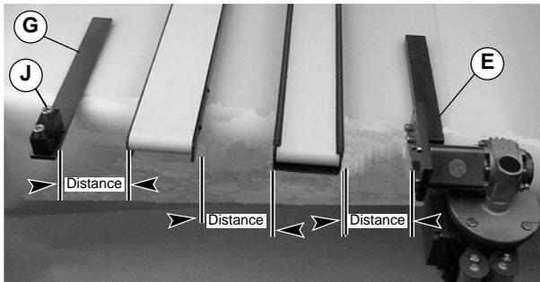
**Step 7:** Properly align and position conveyors between gearmotor support assembly (E) and bearing support assembly (G) as required. Do not secure the conveyors to the mounting surface.
