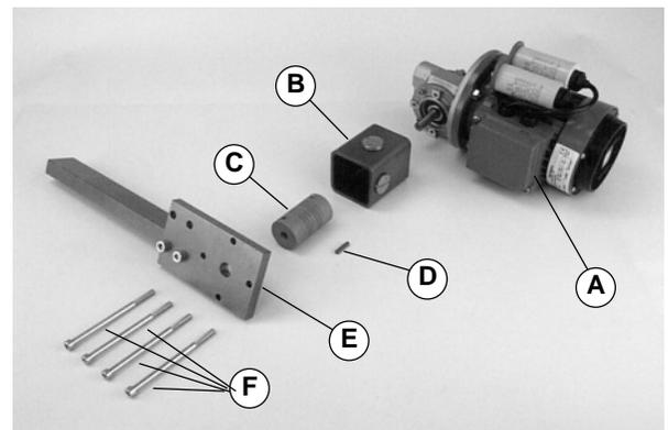
**Step 3:** Build gearmotor assembly as shown. Tighten screws (F) with 50 in-lb (5.6 Nm) of torque.
