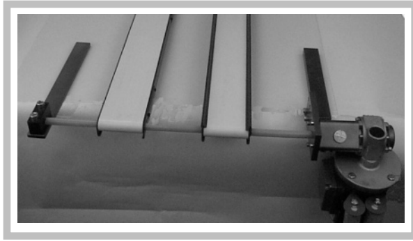
Typical Two Conveyor Gang Drive Mount
