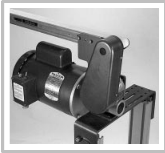
Completed Bottom Mount Package, position "D" shown (Cleated Belt Conveyor Mounting Similar)
