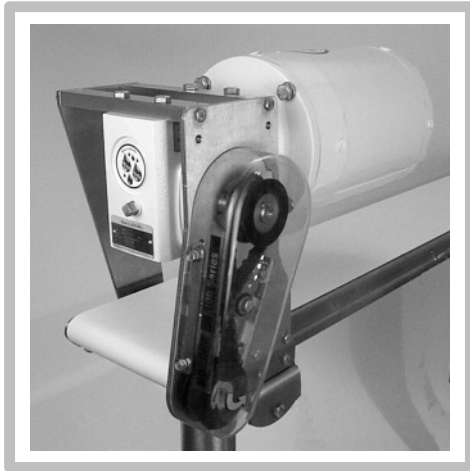
Completed Top Mount Package, position "A" shown (Cleated Belt Conveyor Mounting Similar)
