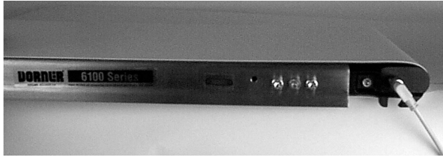
Motion Sensor Installed in 6100 Series Industrial Conveyor Tension End Tail Plate
