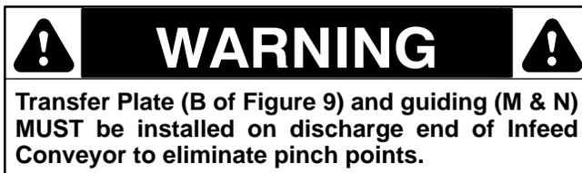
13. On the discharge end of the infeed conveyor (A of Figure 9):
