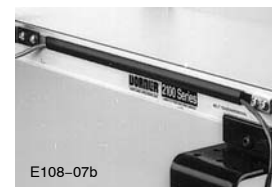
Figure 7: T-slot Cover Strip Mounting Details
