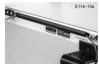
Figure 10: Closure Strip Mounting Details
