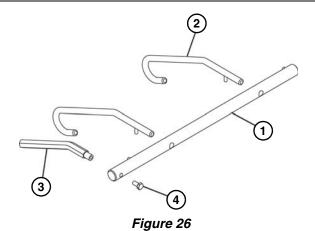
1. Slide the belt lift pivot bar (**Figure 27, item 1**) through the designated holes in the frame.
