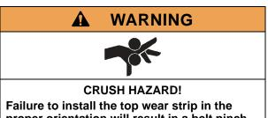
proper orientation will result in a belt pinch point. Exposed moving parts can cause serious injury.
