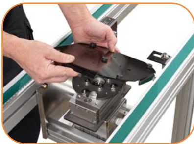
STANDARD FEATURE: Breakaway Top Plate
