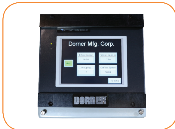
HMI Interface Setting, Spacing and Speed
