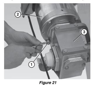
6. Detach the motor (Figure 22, item 1) from the gear reducer (Figure 22, item 2).
