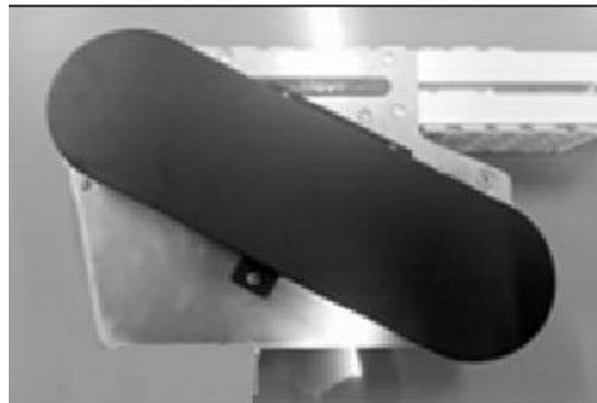
Motor cover for the bicycle chain transmission
