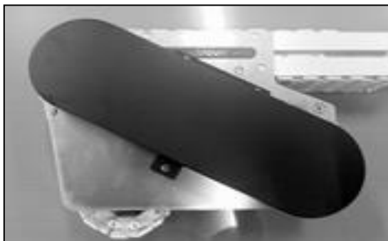
Drive Cover to cover the chain slag for suspended drive unit
