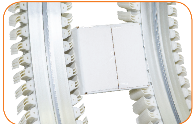
Products are wedged between opposing conveyors
