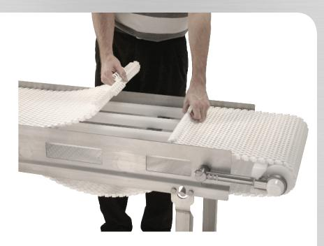
sliding it off the frame, removing the wear strips on the frame that support the belt, and sliding the tails off — it's that easy. This quick process provides complete access to the frame for cleaning. Being able to rapidly disassemble a conveyor, sanitize it and put it back into service increases OEE, not just for the conveyor, but for the entire line.
