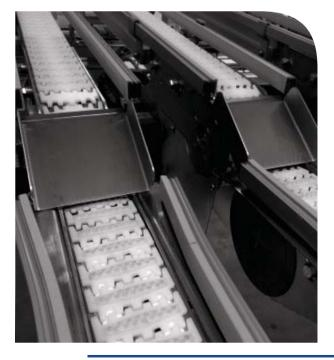
UOM: 5 Meter / box Application: Suitable for transport product in slope > 5 ° but ≤ 30 ° without accumulation.
