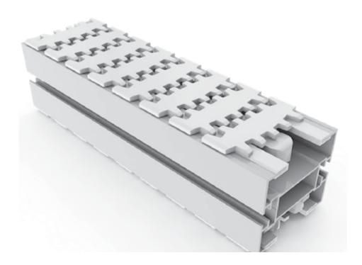
Variety of chain type suitable for wide range of applications either horizontal or vertically product transportation. Capacity higher than FK and FS. The maximum product width to be conveyed can be referred to guide rail assembly pages.
